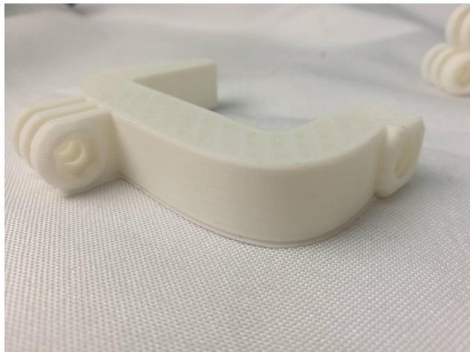
Set the seam position of the printing model as the specified position. The printing model effect is as follows:
