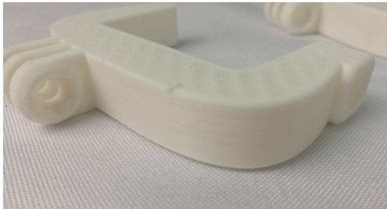
The setting of the printing model is the sharp corner position. The printing model effect is as follows:
