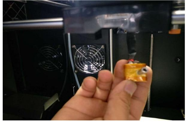
After that, heat the nozzle to 200 degrees, fix the nozzle with a tool such as a pliers, and use a 1.5mm wrench to clear it until the blocked wire is completely cleaned.
