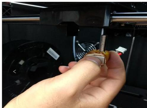
Completely unscrew the two hexagon socket head cap screw at right side, and take out fan and cooling fan.
