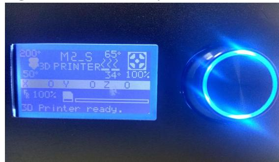
After printer starts heating, LCD would display the real temperature of nozzle and printing platform. At this moment, if needs to perform other operation, users can press the left button to return to stat menu, and heating process will continue at the backstage. If needs to stop the printer heating, users can enter to heating menu and choose "Stop-Heating" .
