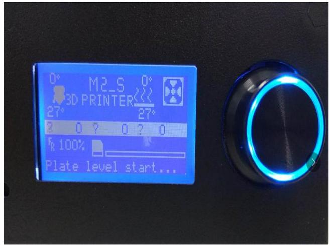
At this point, the printer will enter the following interface. When the printer nozzle moves to a fixed point, start adjusting the spin button on the bottom of the platform and adjust the gap between the platform and the nozzle until the A4 paper has a slight frictional resistance when sliding. After adjustment, click the spin button to enter the next adjustment point until the four-point leveling is completed (the same level is used for each level).
